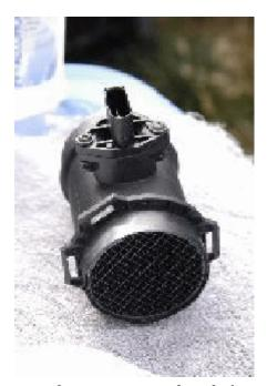
6. Screw clean sensor back into tube
