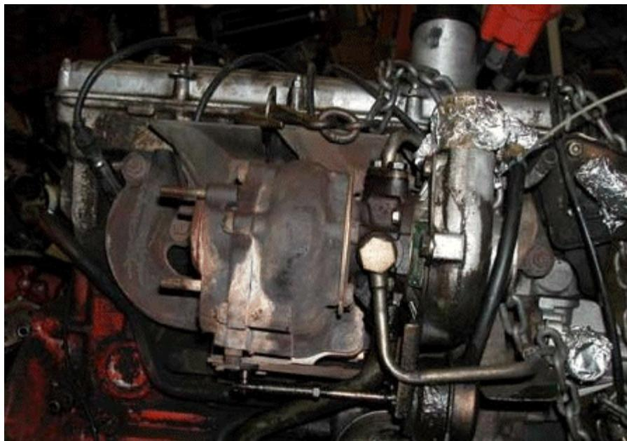
This Mitsubishi TD05 is on a 1987 B230FT and was used in 1987-1989 model years. Note the wastegate is bolted to the exhaust
