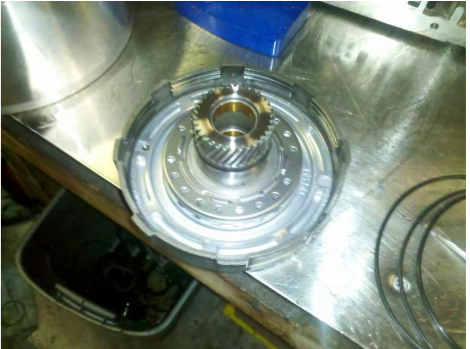
Overdrive overhaul (lol): overdrive unit with OD clutches removed:
